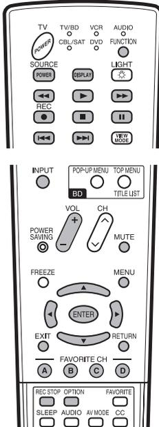
You can operate AQUOS LINK-compatible devices with the remote control unit when the **FUNCTION** of the remote control unit is set to TV/BD.
