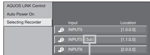
When an AQUOS LINK-compatible audio system or other equipment is connected between the TV and recorder, "Sub" is displayed.
