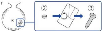
4. Attach the base, and then secure with a screw. Use a coin or similarly shaped object to tighten the screw.
