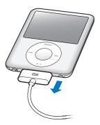
If your Dock connector is larger than the one shown, squeeze both sides of the connector while removing.
