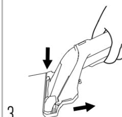
3 To lift the stain, suction up the dirt and cleaning solution by applying downward pressure on the front of the cleaning tool and pulling towards you. Repeat as needed.
