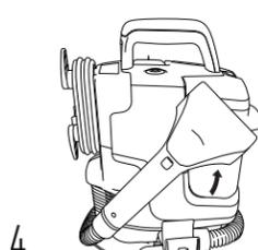
4 Unwrap hose from unit. Select preferred tool and make sure it is attached securely.
