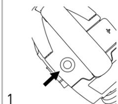
1 Plug power cord into electrical outlet. Press Red Button on top of unit to turn ON.
