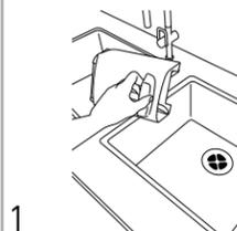
1 Press TANK RELEASE button then lift lid off for emptying and rinsing. Clean water will help remove dirt & debris from the tank. Let air dry before reinstalling.
