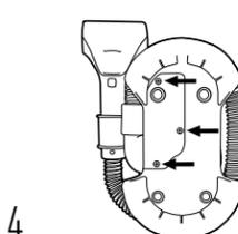
4 Access the hose for cleaning by removing the three screws on the bottom of the carpet cleaner. Once removed, slide the piece away and rinse.
