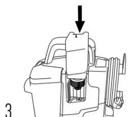
3 Replace and tighten cap. Slide the Tank back into the unit to secure the tank.
