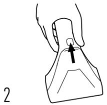
2 Rinse hand tool under faucet. Remove nozzle cover by pressing release button on top.
