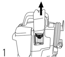
1 Remove Solution Tank from the side of the unit, then remove the cap.
