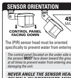
The control panel (located on the under side of the sensor) **MUST** face down toward the ground at all times to prevent water from entering and damaging the unit.
