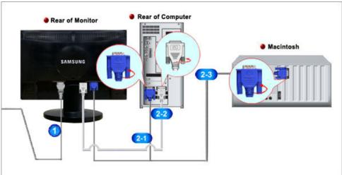
Onnect the power cord for your monitor to the power port on the back of the monitor.
