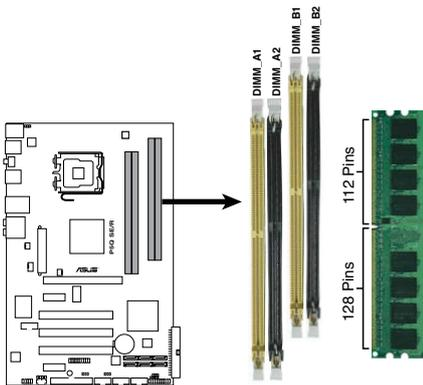
**P5Q SE/R 240-pin DDR2 DIMM Sockets**
