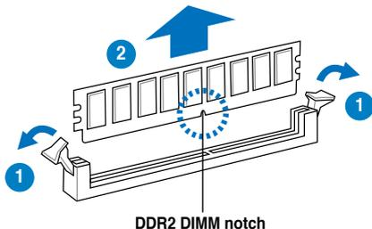
2. Remove the DIMM from the socket.
