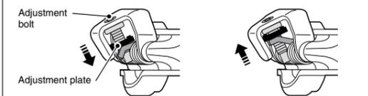
If the adjustment plate is at the strongest or the weakest position, do not turn the adjustment bolt any further.
