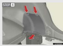
Remove the 12-volt battery maintenance cover.
