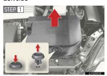
Remove the power control unit cover.
