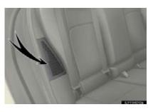
There is an air intake vent on the side of the rear right seatback for the purpose of cooling the hybrid battery (traction battery). If the vent become blocked, the hybrid battery may overheat, leading to a reduction in hybrid battery output.
