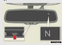
To turn the compass on or off, press the "AUTO" button for more than 3 seconds.
