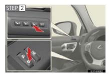
Press the desired button (1, 2 or 3) to recall the position. Then, while keep pressing the button, press the driver's door lock switches (either lock or unlock) until the signal beeps.
