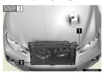
After the hybrid system has cooled down, inspect the hoses and radiator core (radiator) for any leaks.
