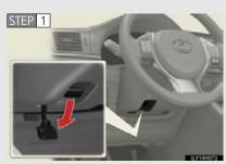
Hold the steering wheel and push the lever down.
