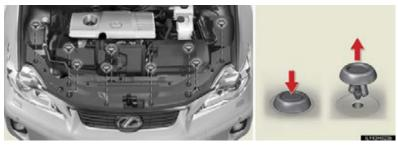
■ Installing the clips
