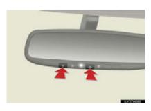
Press and hold the 2 outside buttons shown in the illustration for 10 seconds until the indicator light flashes
