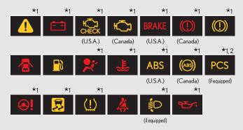
\*1: These lights turn on when the "POWER" switch is turned to ON mode to indicate that a system check is being performed. They will turn off after the hybrid system is on, or after a few seconds. There may be a malfunction in a system if a light does not come on, or if the lights do not turn off. Have the vehicle inspected by your Lexus dealer.
