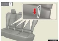
Open the fasteners on the lower part of the seatback.
