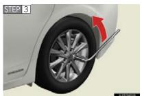
Slightly loosen the wheel nuts (one turn).
