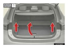
Remove the side deck boards and open the center auxiliary box.
