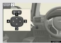
To adjust the mirror, press the switch.
