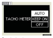
Press the "DISP" switch and select the desired setting, and then press and hold the "DISP" switch.
