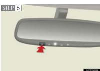
Press and hold the programmed HomeLink® button (located inside the vehicle) for 2 seconds and release it. Repeat this sequence (press/hold/release) up to 3 times to complete programming.
