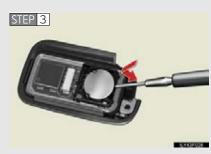
Remove the depleted battery.
