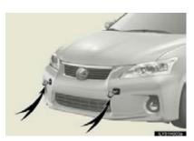
If a tow truck is not available in an emergency, your vehicle may be temporarily towed using a cable or chain secured to the emergency towing eyelet(s). This should only be attempted on hard surfaced roads for short distances at under 18 mph (30 km/h).
