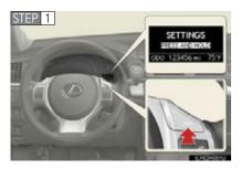
Press the "DISP" switch to display the "SETTINGS" screen while the vehicle is stopped, and then press and hold the "DISP" switch to display the customize mode screen.
